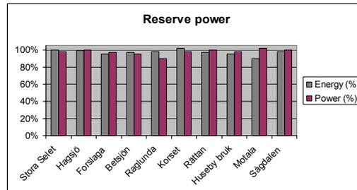
The energy capacity can be measured by discharging and charging the battery, but in reality this is not often used. Usually the battery is simply replaced after a certain period of time. The uncertainties concerning capacity reduce reliability and increase costs. In order to secure high reliability, the batteries are replaced long before the problems may occur. In diesel generators the effect as well as the stored fuel can be easily measured.
