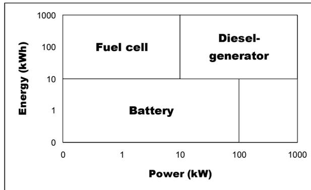
When both large effect and energy storage are required, diesel generators are the most competitive alternative.
