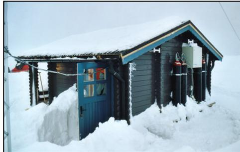
During winter 2004, a 50 W-fuel cell unit was tested in an industrial area close to Stockholm. The unit was placed in a non-heated outdoor cabinet. The temperature during the test period dropped to -20 °C. The energy storage consisted of 12 standard bottles of industry quality hydrogen, so called Europall (totalling 120 kWh electricity).
