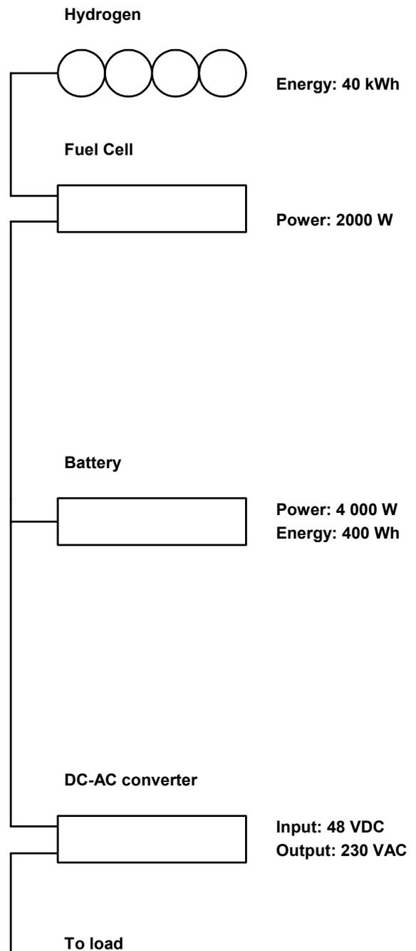
Cellkraft offers complete systems based on the building blocks described in this fact sheet.
