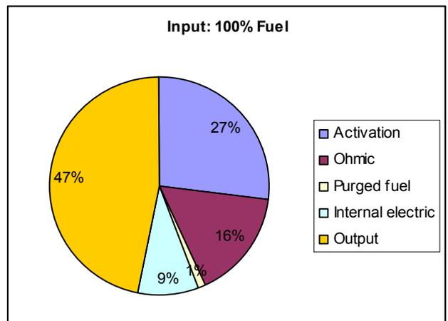
Cellkraft S-1000 has an efficiency of 47 % at 1000 W net output. That corresponds to a hydrogen consumption of 12,7 nl/min.
